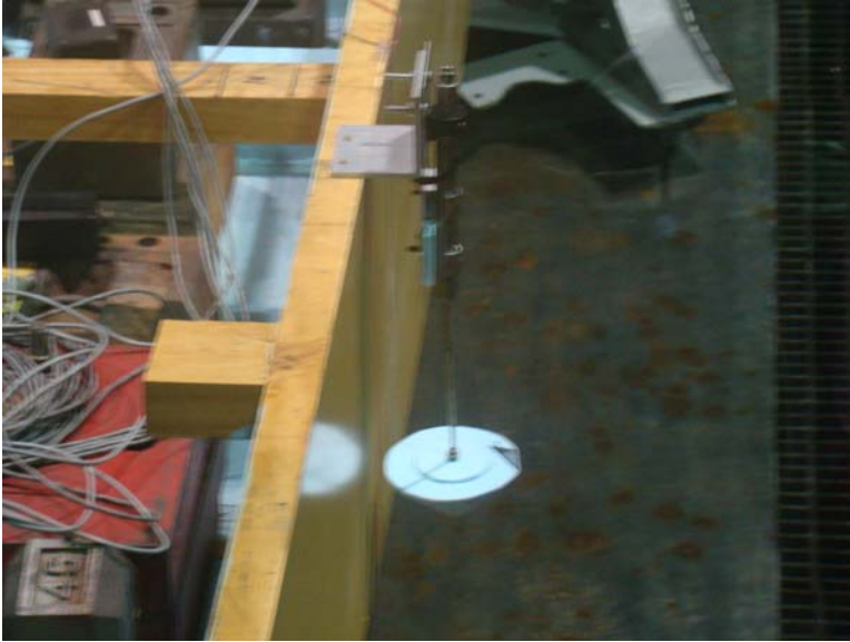
Figure 8: The final wave profiler hooked up and attached to the side of the model.
